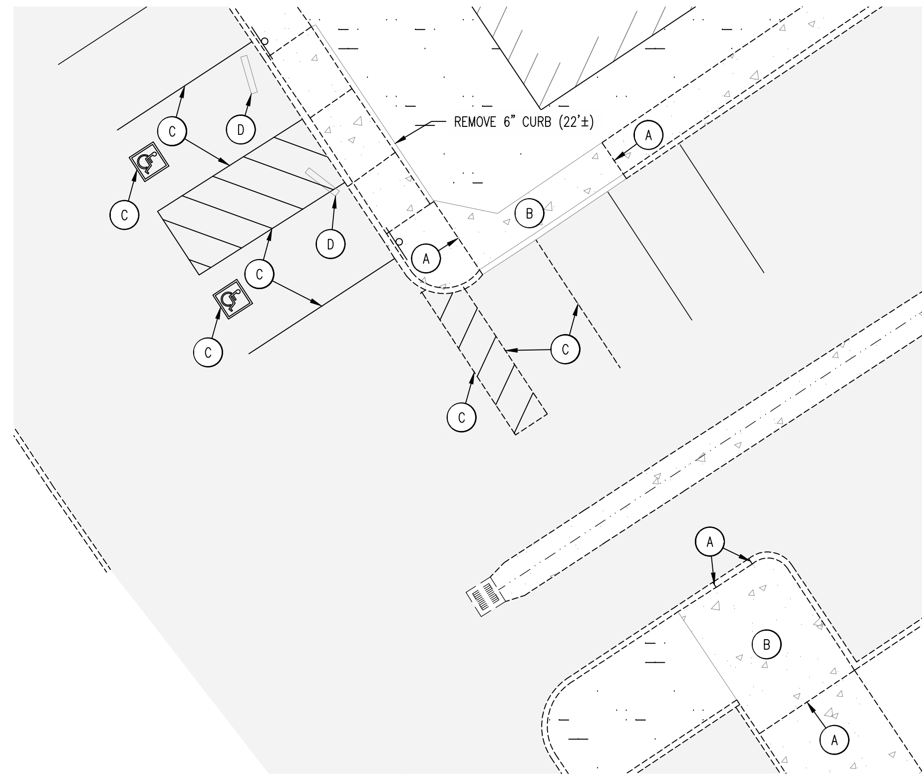
DEMOLITION PLAN SCALE: 1" = 10' A C2.0
